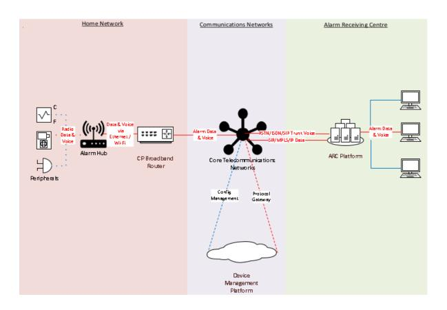
It should be noted that, whilst connecting a digital alarm to a single broadband router only connection is preferable to connecting an analogue alarm to a broadband router, there are risks to this type of solution as it relies entirely on the service user's internet connectivity set-up and power to operate successfully.
