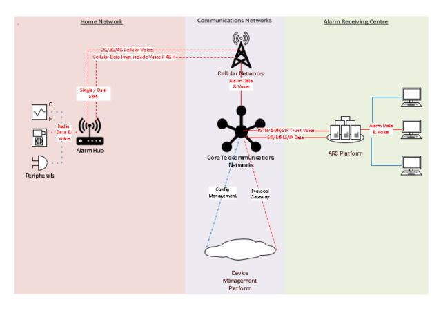
It should be noted that when the solution is reliant on a single SIM card with a single communication method to the ARC, the risk of solution failure is higher than when there is either a combined SIM/Broadband option, a multi-SIM option or a single SIM/multi-IMSI option
