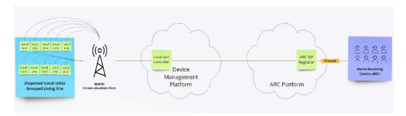
b. The dispersed digital Local Units are registered directly with the Alarm Receiving Centre (ARC) platform SIP registrar which enables the ARC platform to have visibility of all of the scheme alarm devices connected to it. In this instance, each scheme Local Unit (alarm device) would require its own account (username / password etc...) on the ARC SIP registrar.
