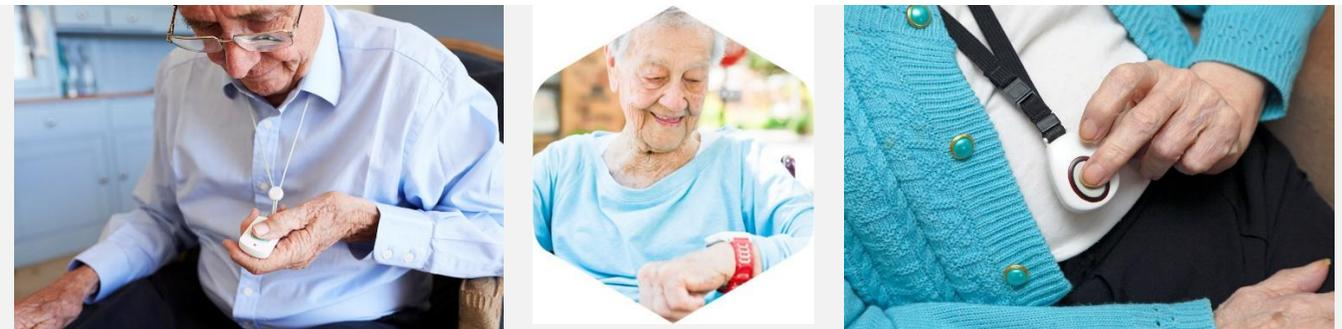
Commonly, a telecare alarm trigger is worn on the body, usually around the neck, or on the wrist. The person presses the button on the trigger to get help, especially if they fall and can't get up. When the TCP receives an alarm, they can talk to the person through a speaker. Many other types of telecare and telehealth devices are also available – go to 'Find TEC Services' at <https://www.tsa-voice.org.uk/>.
